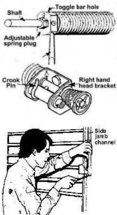
1/ With the door in the closed position, insert the supplied crook pin through the shaft in the right hand head bracket to retain the spring tension as described above.
