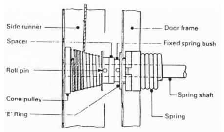
5/ Remove the hollow roll-pin from each cone using a 4mm pin punch. (Our Ref: APL0040) Slide both cones off the spring shaft.
